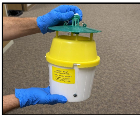
Figure 11: Remove the basket from the funnel.
