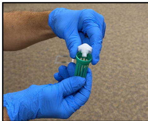
Figure 12: Remove cap from the lure basket.
