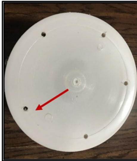
Figure 40: Plastic bucket trap with drilled holes (see red arrow)
