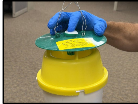
Figure 18: Attach the lure basket to the funnel. Photo credit: Christopher Pierce, USDA (2025)
