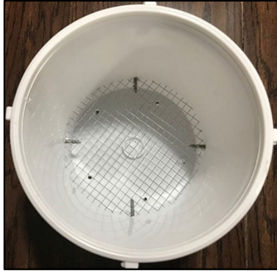
Figure 42: Screw placement for mesh screen Photo credit: Christopher Pierce, USDA (2025)
