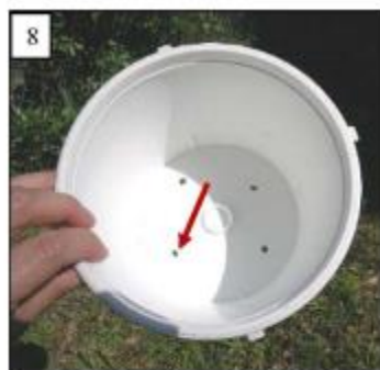
Fig. 8. Bucket with four drilled holes.
