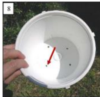
Fig. 8. Bucket with four drilled holes.
