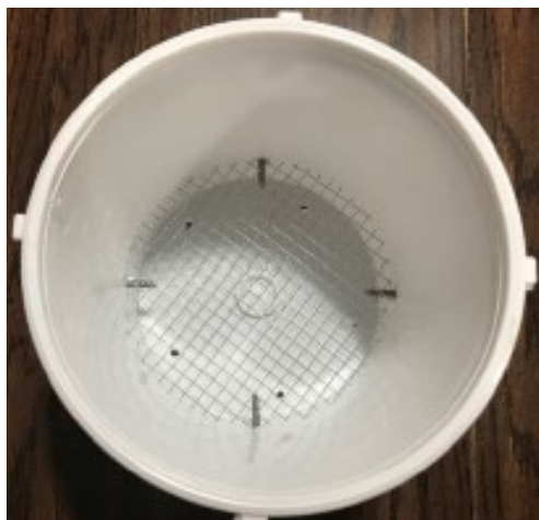
Figure 16. Wire mesh screen placed on machine screws inside bucket trap
