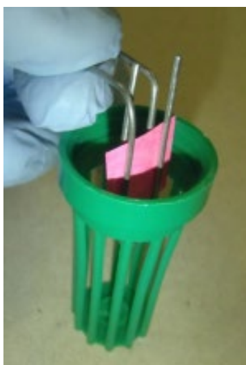
Figure 5. Laminate lure in paper clip inside lure basket
