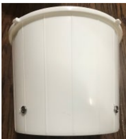
Figure 15. Machine screws shown one inch from the bottom of the bucket trap (outside)
