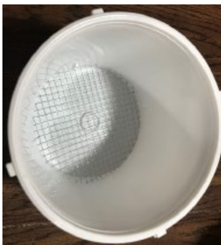
Figure 13. Wire mesh screen in bucket
