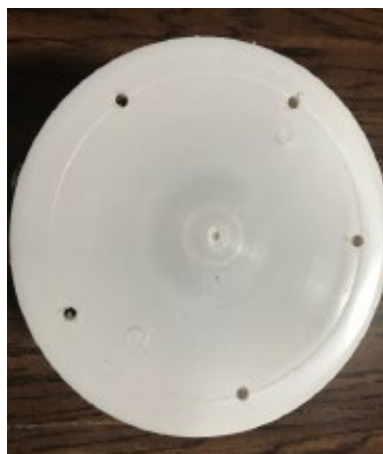
Figure 11. Bucket with five holes drilled in the bottom
