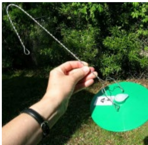
Figures 8 and 9. Wire handle attached to trap lid
