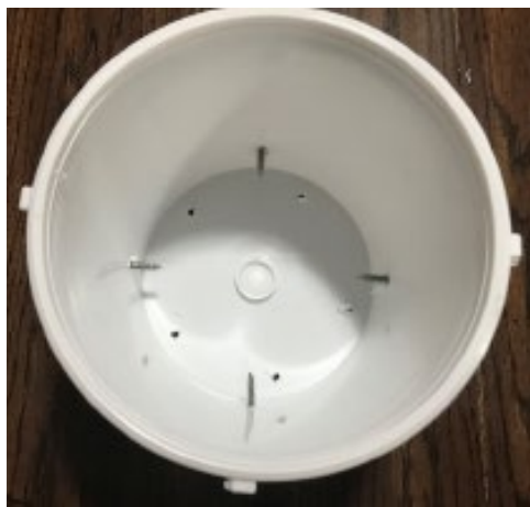
Figure 14. Machine screws placed equal distance from each other and around the bucket trap (inside)
