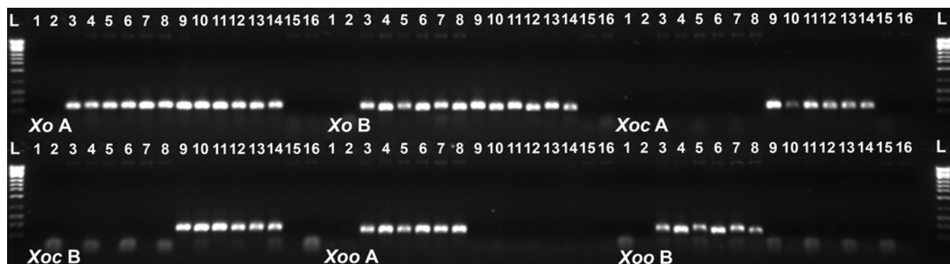
Fig. 2. Conventional polymerase chain reaction screen showing specificity of 12 computationally designed primers to amplify Xanthomonas oryzae (panels XoA and XoB), X. oryzae pv. oryzicola (XocA and XocB), or X. oryzae pv. oryzae (XooA and XooB). Primers screened in panel XoA were Xo2207 (324 bp) in odd lanes and Xo3756 (331 bp) in even lanes; panel XoB: Xo2967 (336 bp) odd lanes and Xo1321 (304 bp) even lanes; panel XocA: Xoc3866 (335 bp, later redesigned to produce 691-bp fragments for the multiplex) odd lanes and Xoc2071 (329 bp) even lanes; XocB: Xoc3864 (377 bp, later redesigned to produce 945-bp amplicons for the multiplex) odd lanes and Xoc3863 (360 bp) even lanes; XooA: Xoo80 (162 bp) odd lanes and Xoo4009 (302 bp) even lanes; XooB: Xoo2976 (337 bp) odd lanes and Xoo3350 (300 bp) even lanes. The bacterial strains screened are in this order: lane L, 1-kb Plus DNA Ladder; lanes 1 and 2, negative control; lanes 3 and 4, X. oryzae pv. oryzae MAFF311018; lanes 5 and 6, X. oryzae pv. oryzae NXO588; lanes 7 and 8, X. oryzae pv. oryzae A3857 (110); lanes 9 and 10, X. oryzae pv. oryzicola BLS256; lanes 11 and 12, X. oryzae pv. oryzicola BLS99; lanes 13 and 14, X. oryzae pv. oryzicola BLS483; and lanes 15 and 16, X. campestris pv. phleipratensis . Primer sequences are listed in Table 2.
